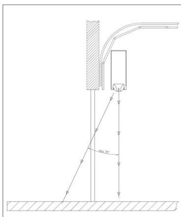
The air curtain system screens a room against cold air and draughts that impact on the door from outside. In the case of high outside pressure (wind pushes towards the inside) a higher volume of air (e.g. level 5) should be selected on the controller to counteract the pressure.
