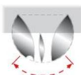
The air discharge angle of the nozzle can be finely adjusted by hand or by means of grids. To obtain maximum screening the nozzle must be directed according to requirements.
